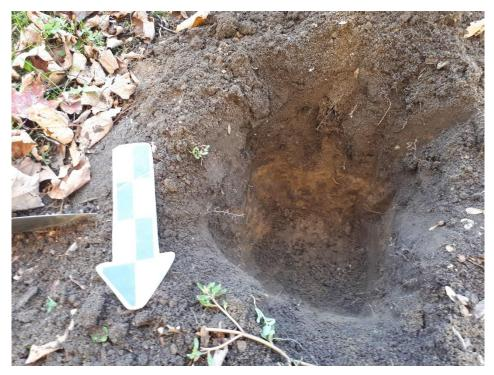
Image 28: Open Test Pit showing soil stratigraphy.
