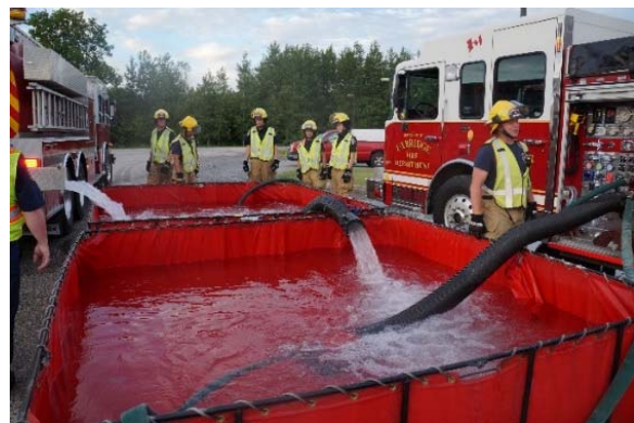
Uxbridge Firefighters participating in a joint rural water supply exercise with Whitchurch-Stouffville Fire & Emergency Services. Shown is WSFES Tanker 514 supplying water to UFD Pumper 71.
