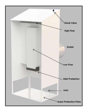
**Figure 2 HydroDome Internal Components**
