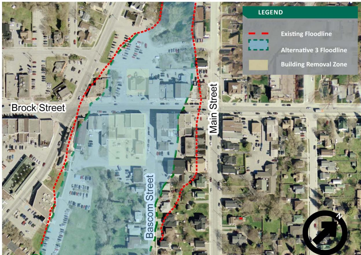
Figure 14. Modeled floodline resulting from Alternative Solution #3
