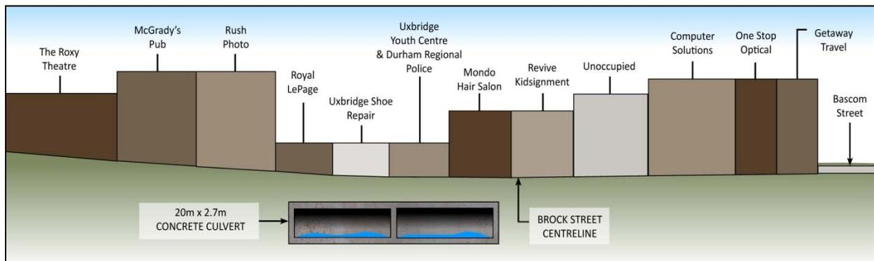
**Figure 9. Conceptual illustration of Alternative Solution #1**
