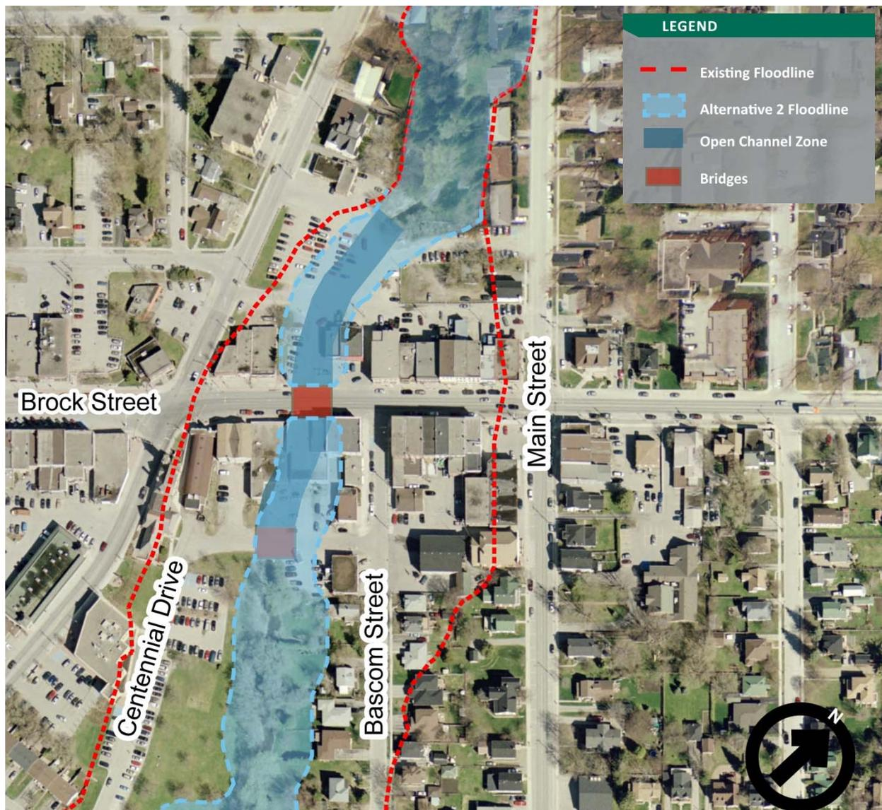
Figure 12. Modeled floodline resulting from Alternative Solution #2
