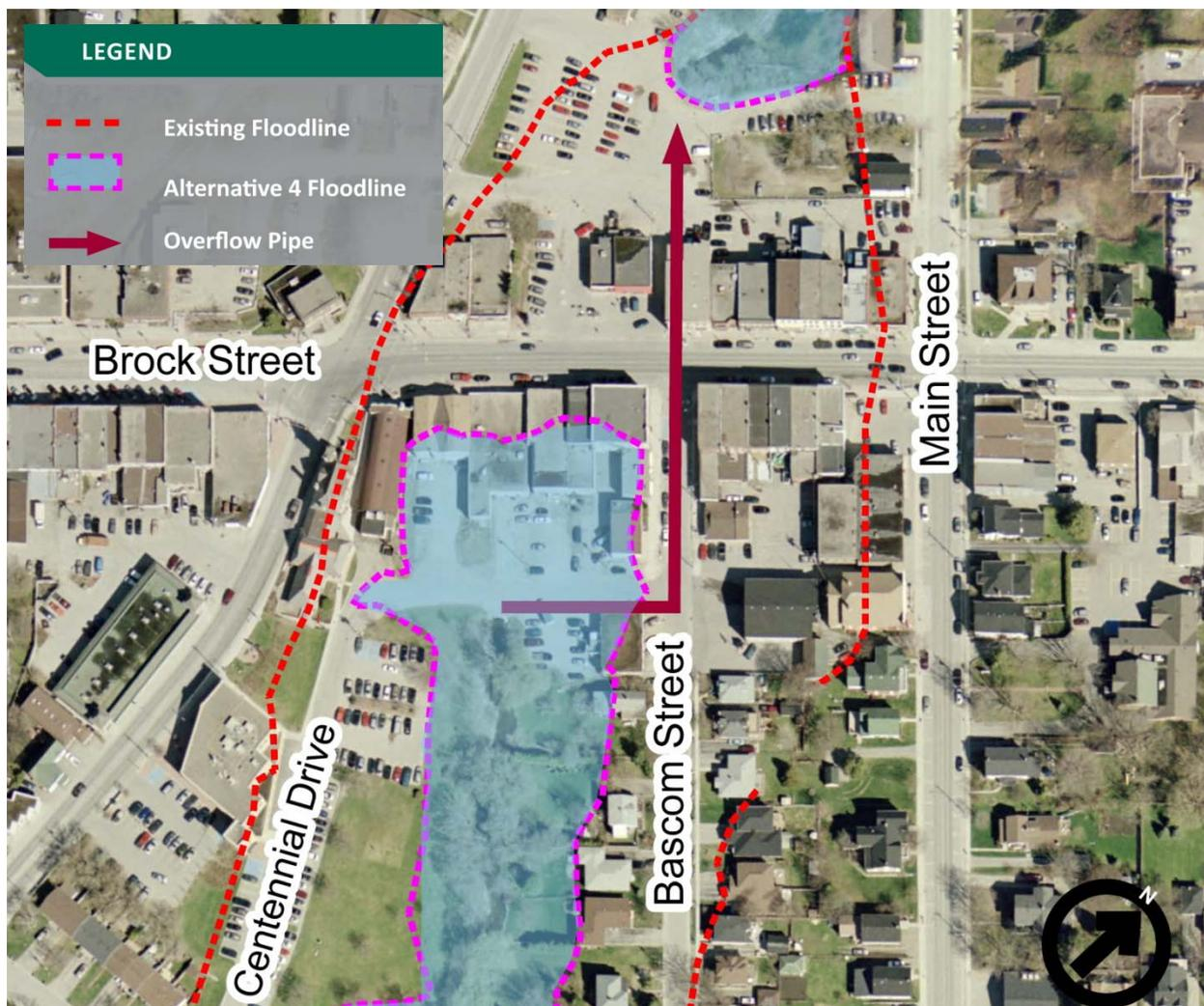
Figure 15. Modeled floodline resulting from Alternative Solution #4
