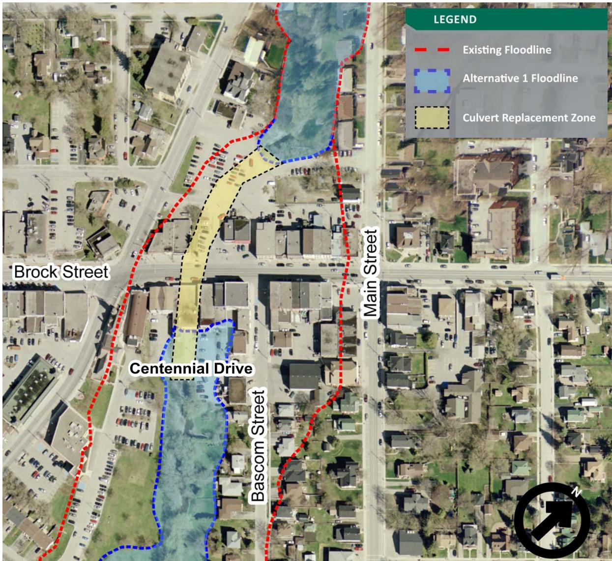
Figure 10. Modeled floodline resulting from Alternative Solution #1
