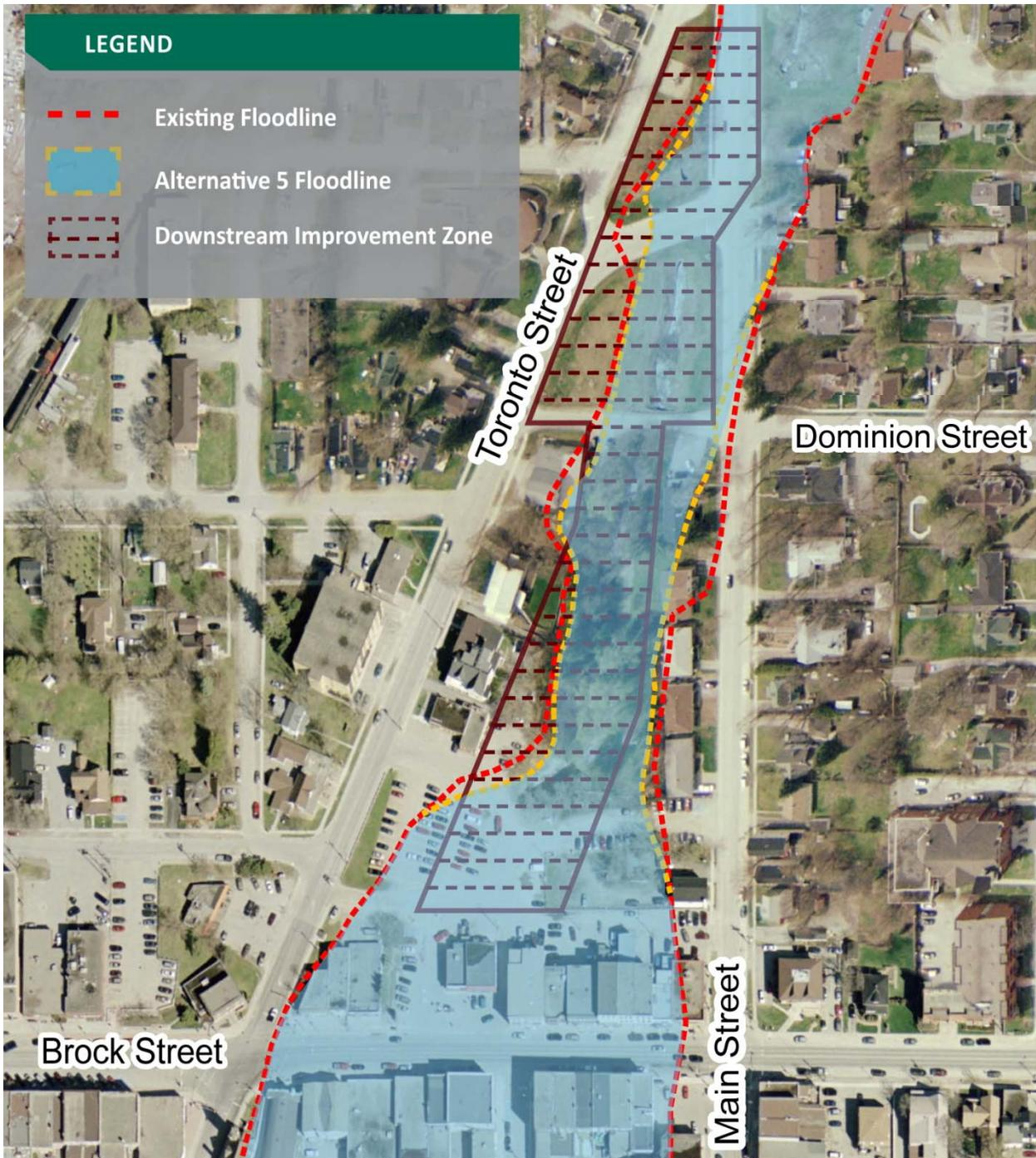
Figure 16. Modeled floodline resulting from Alternative Solution #5
