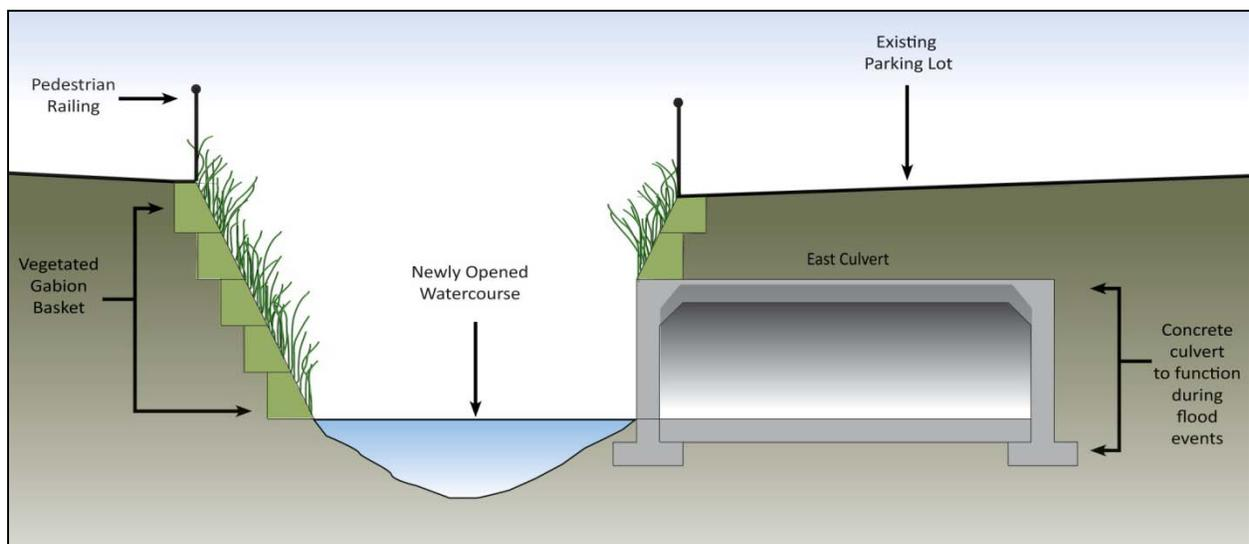
**Figure 28. Conceptual cross-section of the proposed open channel (cross-section B-B)**
